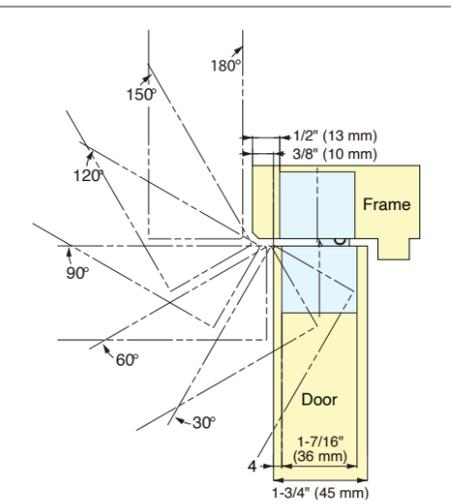
The example drawing shows the case that there is a step of 10 mm between the door and the frame.
