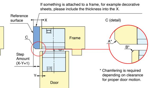
Available on doors which are not aligned flush to the wall or frame.
