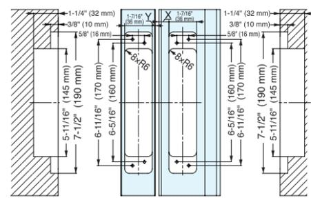
Please drill prepared holes for the tapping screws if the optional jig (HES3D-W190-TMP) is not used.
