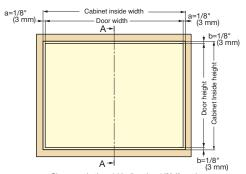
a: Clearance in the width direction 1/8" (3 mm)
